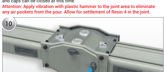
Install the level check pipe to opposite upper port. After level pipe is installed, proceed to injecting the Resin 4 into the joint. Continue the filling process until you see Resin 4 present inside the level pipe. If Resin 4 is present in the transparent pipe and no settlement is observed, that is an indication the joint is full and caps can be closed at this time.
